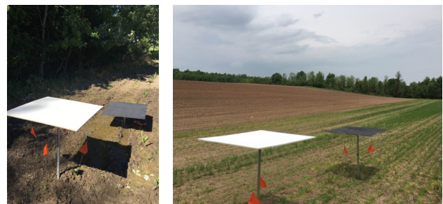
Figure 2. Calibration targets can be impacted by nearby trees (or buildings) and clouds
