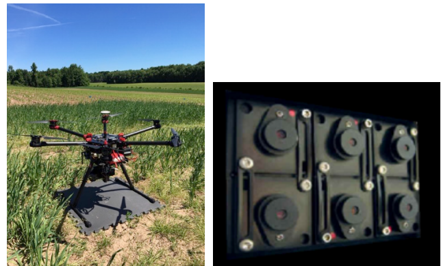
Figure 1. An unmanned aerial system prior to an imaging run and a multispectral sensor
