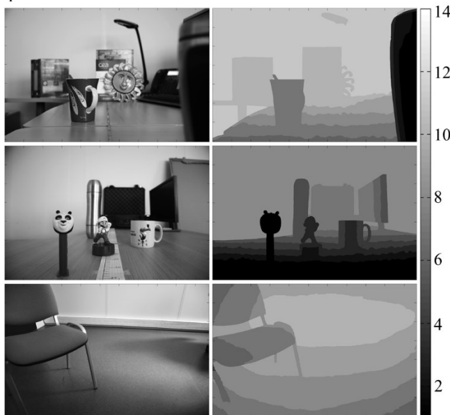
Figure 7. Experimental scenes (left) and the corresponding ground-truth depth maps with their depth index scale (right). The darker, the nearer.
