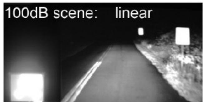
Figure 1. Dynamic Range Gap artifact – linear image with saturation
