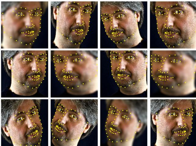
(b) Sample augmented training images with ground truth landmark points annotated. Bounding box random expansion, random rotation and random blurring are applied.
