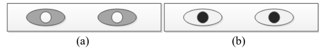
Figure 5. NIR image characteristics of the eyes area. (a) genuine eyes; (b) printed spoof eyes.
