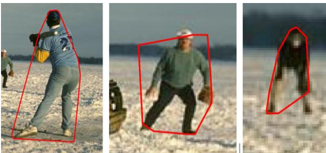
Figure 10 Superpixel human detection results. It shows ability of the superpixel algorithm to detect foreground information in various resolutions.
