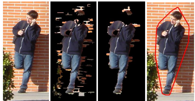
Figure 7. The super pixel human detection pipeline. The superpixels are found in the imagery and matched to corresponding background and foreground patches. Small unconnected superpixels are removed due to no relevance to the foreground object. A convex hull is placed over the group of superpixels, creating a segmented object.
