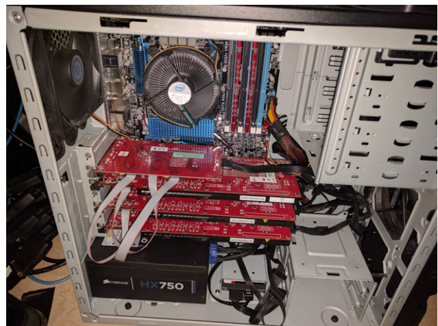
Figure 4. Computer system driving a single wall with three graphics card that are synced with all other computers.
