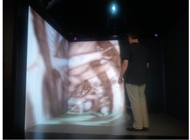
Figure 8. User exploring a volume rendering of a CT angiogram data set in an immersive environment.
