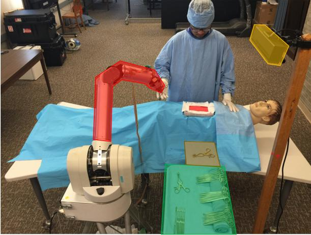
**Figure 2.** Illustration of the system. The highlighted regions are mayo tray (green), recognition pad (brown), Kinect (yellow) and robotic arm (red).
