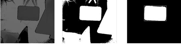
**Figure 4.** Mayo segmentation procedure. (left) raw input depth image  $I_D$  from Kinect; (middle) foreground mask  $M_{fg}$  generated from Otsu's threshold; (right) mayo mask  $M_{mayo}$  generated from contour examination
