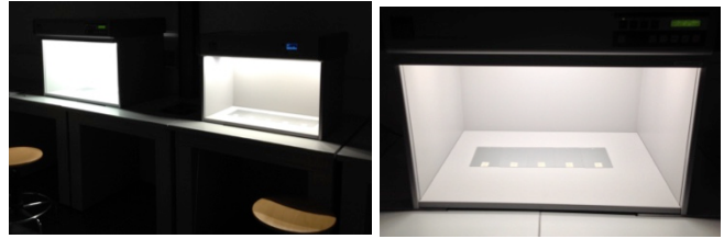
Figure 1: left: the two lighting booths used during the experiment, right: the fluorescent lighting booth
