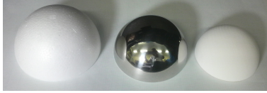
Figure 6. A photograph of the hemispheric objects—styrofoam (left), specular stainless steel (middle) and matte-painted wood (right).
