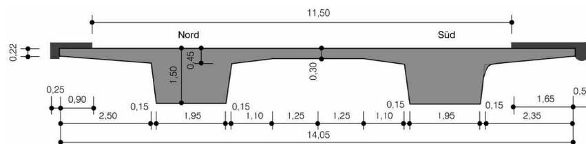
Figure 2: Schematic representation of the cross of the example calculation in [3].
