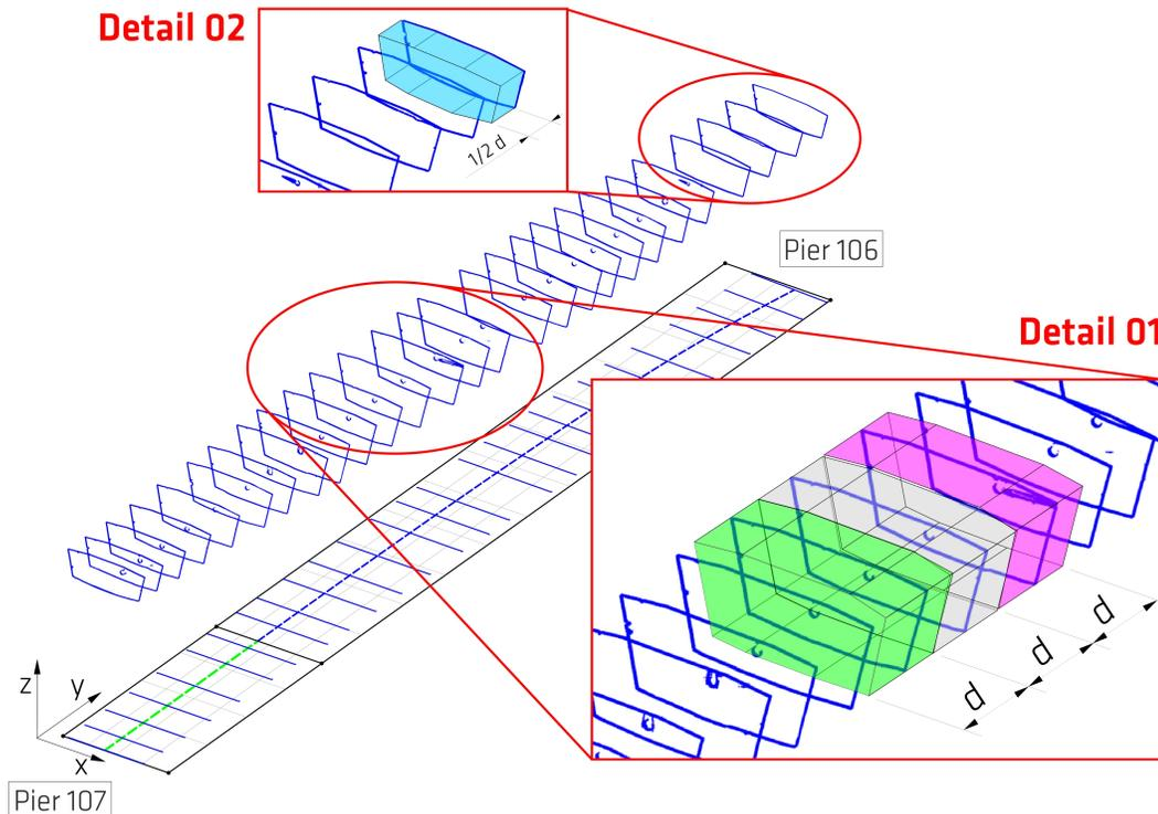
Figure 17: Segmentation of the volume elements for the approximate calculation of the internal volume.
