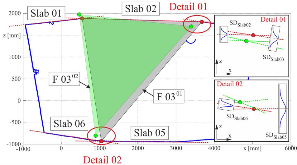
Figure 15: Schematic representation of the influence of the displacement of the calculated intersection points on the newly developing surface (green).
