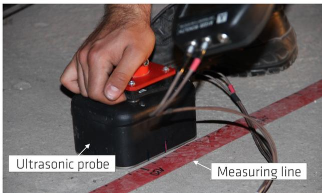
Figure 12: Determination of the thickness of the component by ultrasonic echo measurements with an offset of the measuring points of 5 cm.
