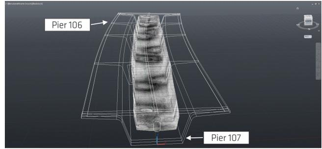
Figure 7: Representation of the point cloud measured by the LiDAR method faded into the bridge model drawn with CAD.
