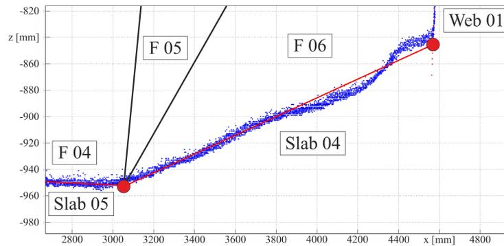
Figure 10: Representation of the surface of the concrete (blue points - LiDAR) at a selected typical position of the structure (figure from [5]).
