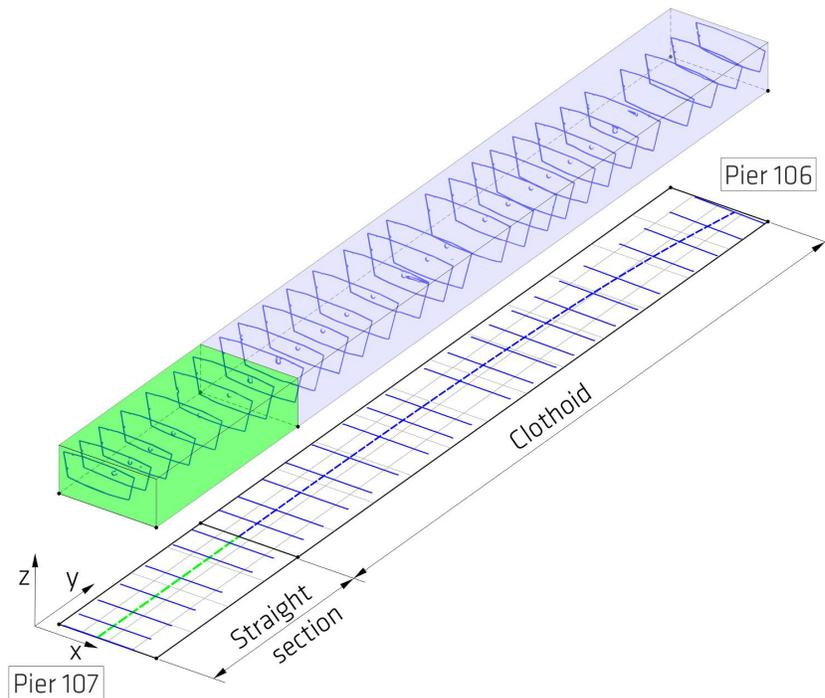
Figure 8: Illustration of the 27 segments extracted from the point cloud at the positions where NDT measurements were carried out. The section of the investigated structure is divided into a straight section (green section) and a clothoidal section (blue area).
