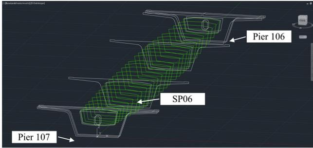
Figure 6: CAD drawing of various cross sections of the bridge (white lines). Green colored lines represent the 27 positions of the NDT measurements [5].
