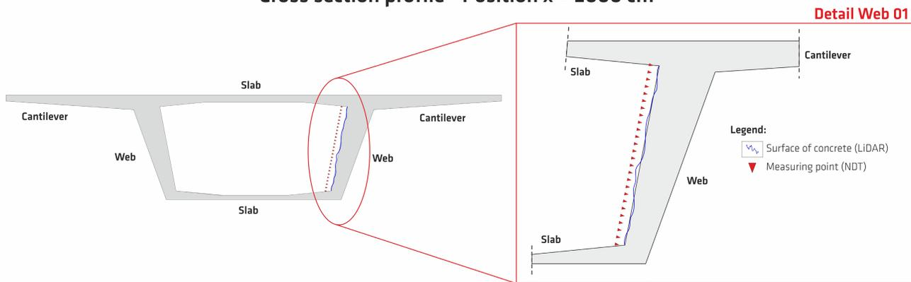
Figure 11: Schematic representation of the inner area of the hollow box and the available conditions during the measurement with the NDT methods.
