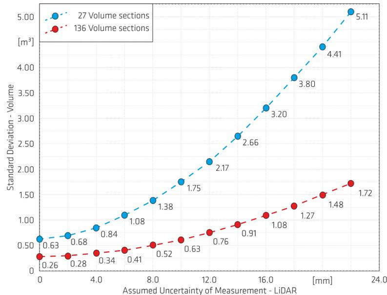
Figure 19: Estimation of the influence of the uncertainty of measurement of the LiDAR method on the calculated internal volume of the bridge element for two cases of the segmentation of the volume.
