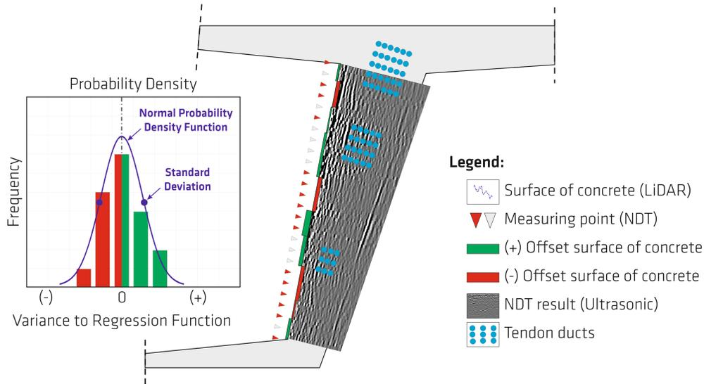
Figure 13: Schematic representation of the real conditions in the determination of the constructional thickness of the hollow box girder by NDT measurements and the resulting consequences.
