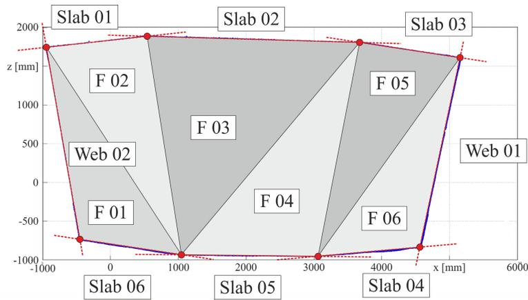
Figure 9: Results from [5] of a reconstructed cross-section profile by linear regression of the component geometry.
