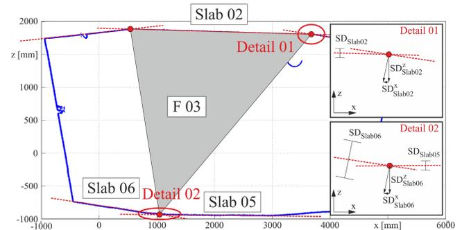
Figure 14: Representation of the straight lines formed by linear regression, giving the related standard deviation for the cross profile SP06 from [5].
