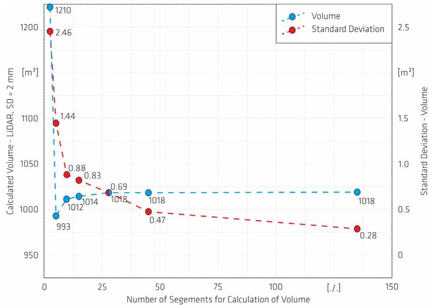
Figure 18: Diagram of the change in the calculated volume and the associated standard deviation as a function of the segmentation of the volume elements with an assumed uncertainty of measurement of  $\pm 2$  mm for the LiDAR method.
