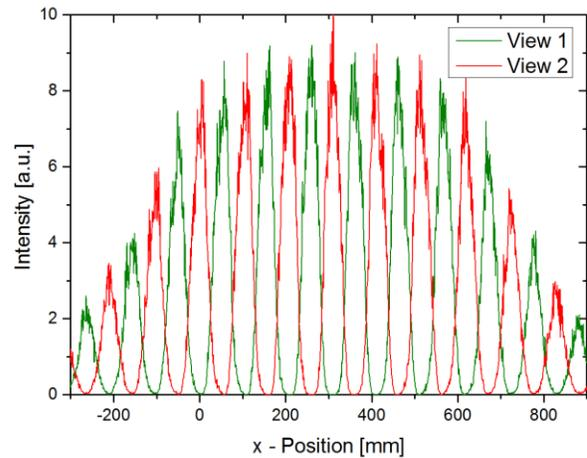
**Figure 3.** Integrated light intensity of the views in 1.2 meter distance to the 3D display, two views separated by green and red color, display width of around 0.6 m, x-position zero is the left edge of the display.
