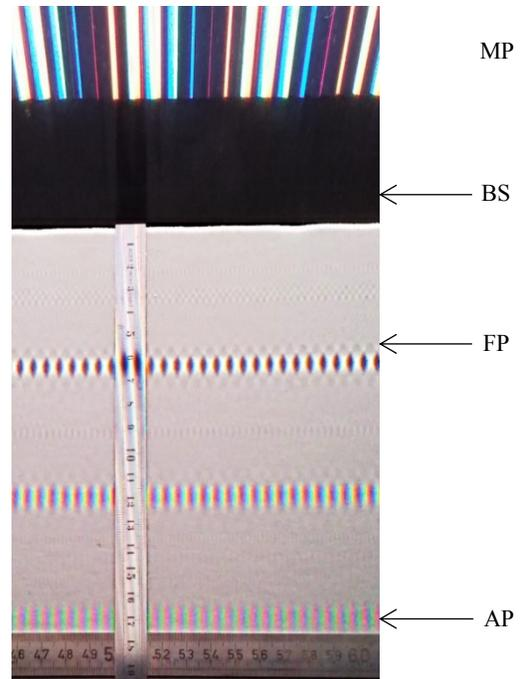
Figure 8. Horizontal light distribution with alternating colored strips in several distances to image splitter  $BS$  and pixel plane  $MP$ , anterior focal plane  $FP$  is barely visible; RGB-pattern is sharply separated in 17 cm distance from  $BS$  at air-image plane  $AP$ .
