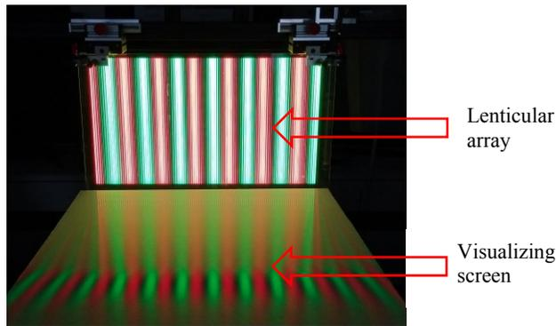
Figure 7. 3D display setup with test content.
