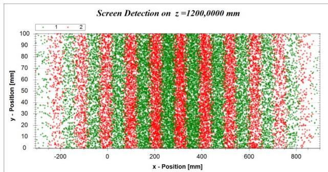
**Figure 2.** Screen detection plane in 1.2 meter distance to the 3D display, two views separated by green and red color, every single Point represents one emitted ray from the pixel plane, display width of around 0.6 m, x/y-position zero is the lower left corner of the display.
