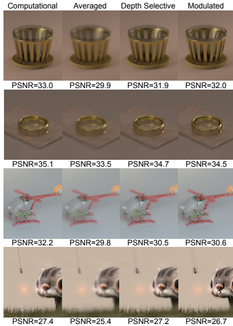
Figure 10. Comparison of 4 reconstruction methods of the light fields representing 4 sample scenes. The “computational” reconstruction refers to the ordinary light field reconstruction, which computes the solution of equation (3), and maps the solution to multiple layers. On the other hand, the “averaged” reconstruction puts the accumulation images on those layers. The other two methods make use of scenes’ depth maps as supplementary information to determine the layers’ weight before fusing the images. The weight is computed for each pixel and for each view direction. The “depth selective” reconstruction fuses accumulation images, while the “modulated” reconstruction fuses modulated accumulation images.
