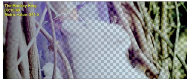
(b) Example of global color mismatch visualized by shuffling square regions of the two views chequerwise
