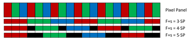
Figure 8. Schematic comparison of stripe widths at periods of 3, 4 and 5 SP .
