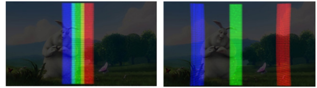
Figure 4. Left: adjacent rendering nodes consume adjacent, slightly overlapping parts of a source view. Red, green, and blue overlays (vertical stripes) represent the areas of the image used by three rendering nodes that drive adjacent optical modules. The areas are slightly overlapping. Right: Rendering nodes that drive optical modules positioned further away from each other use a disjoint set of pixels from the same source view, here the used areas are further away from each other.
