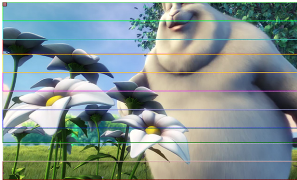
Figure 7. A frame subdivided into horizontal H.264 slices. In an I-frame, these slices can be decoded independently.
