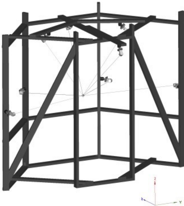
Figure 7. Structure and head-tracking cameras constructed by OBVA lab personnel.
