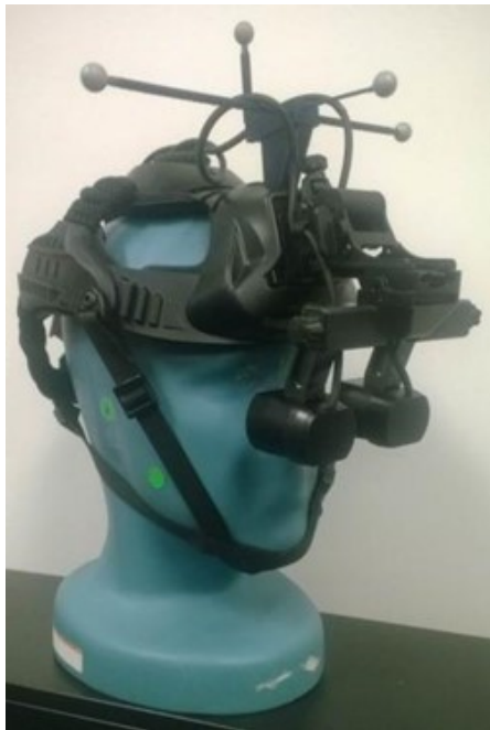
Figure 3. SA-55 HMD configured with 3D printed infrared (IR) reflective rigid body. Photo provided by SA Photonics, used with permission.
