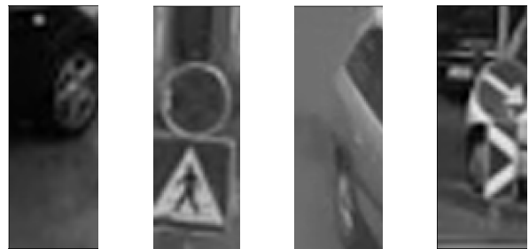
Figure 6. Typical false positives of the HOG detector, which we added to the training set of the CNN detector.
