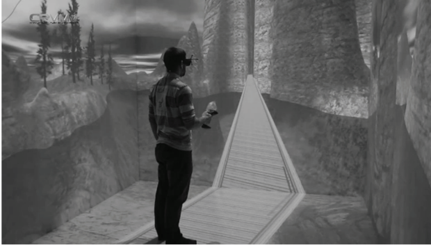
Figure 3. A subject inside a CAVE system, consisting in 4 screens (3 vertical "walls" and a "floor"). This is the most common type of CAVE, using DLP stereoscopic projectors. A few six-sided CAVES exist, favoring a more complete immersion. See for instance [9].
