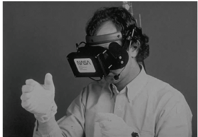
Figure 2. The NASA's First HMD. Note the first "dataglove", used for interacting with the virtual environment.
