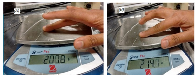
FIGURE 6: TESTING FOR ESTIMATING THE FORCE APPLIED BY THE MIDDLE FINGER (A) AND THE INDEX FINGER (B) WHILE PRESSING A BUTTON
