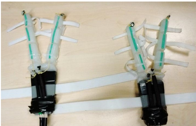
FIGURE 10: FINAL OF THE GLOVE FOR INDEX AND THE MIDDLE FINGER OF LEFT AND RIGHT HAND: ASSEMBLY CONSISTS OF THE SOFT EXOSKELETON, EMBEDDED CHANNELS FOR PASSING THE STRING, MCKIBBEN MUSCLES, AND VELCRO STRAPS TO FASTEN THE GLOVE OVER THE HAND AND FINGERS.
