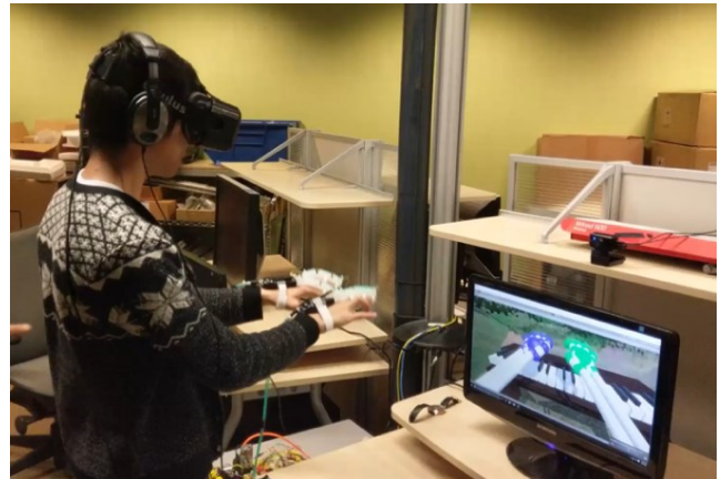
FIGURE 12: USER WEARING THE HAPTIC GLOVE AND OCLUS RIFT AND PLAYING THE PIANO IN VIRTUAL REALITY ENVIRONMENT WITH AUDIO AND HAPTIC FEEDBACK.
