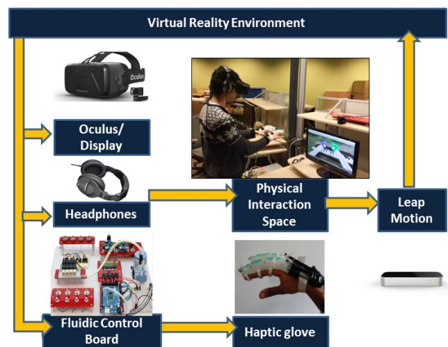
FIGURE 1: THE SCHEMATIC SHOWS THE USER WEARING THE HAPTIC GLOVE AND A HEAD-MOUNTED DISPLAY AND PLAYING THE PIANO IN VIRTUAL REALITY. THE FINGER POSITION IS SENSED BY AN OPTICAL TRACKING SYSTEM (LEAP MOTION). WHEN THE USER PASSES THE VIRTUAL KEY A FEEDBACK IS PROVIDED TO THE GRAPHICS ENVIRONMENT AND A FLUIDIC CONTROL BOARD WHICH ACTUATES THE GLOVE TO PROVIDE A HAPTIC FEEDBACK TO THE USER.
