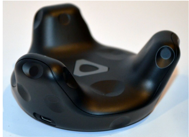
Figure 12. The new Vive Tracker unit. It can be attached to any object that is to be tracked, for instance our head model.
