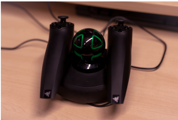
Figure 5. The Sixense Razer Hydra controller provides us a natural user interface for moving objects in 3D space with two hands.
