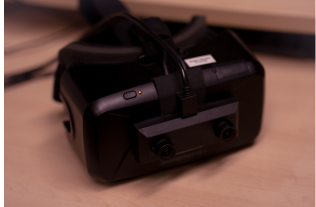
Figure 3. The Ovrvision Pro stereo camera attached to the front of an Oculus Rift DK2.
