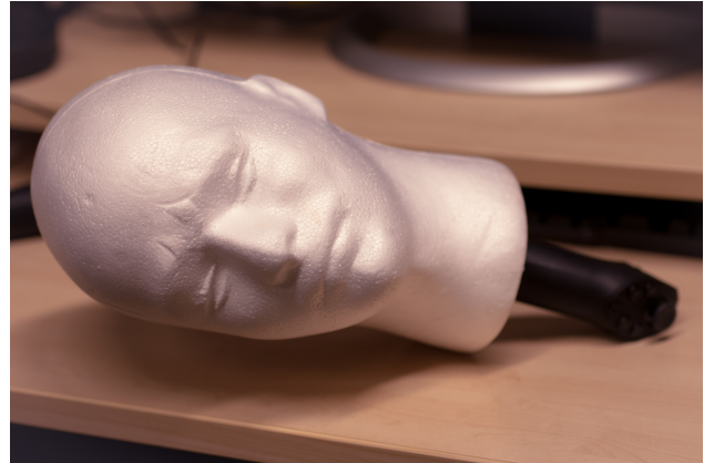
Figure 6. The left hand controller is attached to the physical head model to provide haptic tracking of the head movement as the trainee moves the head.
