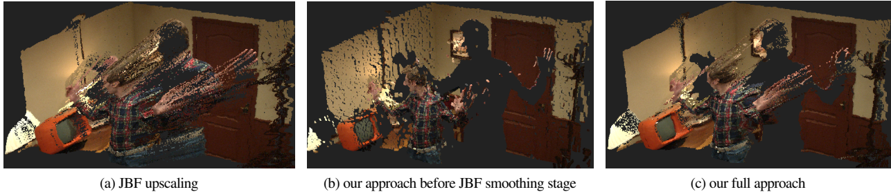
Figure 1: Comparison of resulting 3D point clouds, when using JBF upscaling and our approach with different configurations: the number of flying pixels is drastically reduced. The corresponding depth maps are given in Figure 9.
