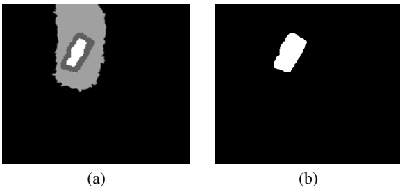
Figure 7. Result of fine segmentation using GrabCut method. (a) The algorithm segment the undetermined region to light and dark gray regions; and (b) The light and dark gray regions are merged to the background and foreground respectively to form the final mask.
