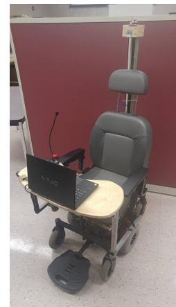
**Figure 2.** Machine Intelligence Laboratory Personal Electronic Transporter (Milpet).
