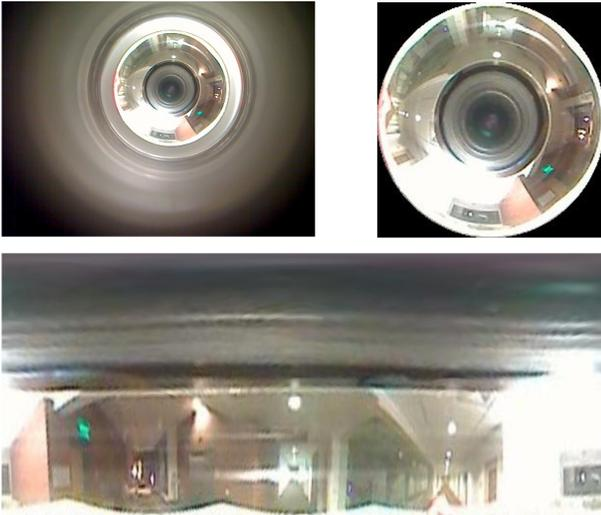
**Figure 7.** Pre-processing steps of the omni-vision camera. Top left is the raw image, top right is the result of centering the image, and bottom is the unwarped image.
