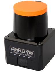
Figure 6. Hokuyo Scanning Laser Range Finder (LiDAR)
