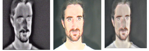
Figure 4. From left to right: thermal image, visible image, fused image by PCA fusion method with Lon illumination.
