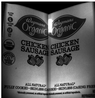
Figure 3. View of POS scanner (with narrow-band red LED), this model has two cameras, creating the two perspectives. The red ink appears white.
