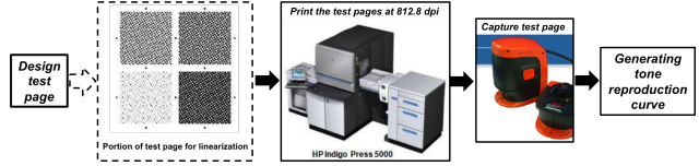
Figure 12. Block diagram of the process for obtaining Tone-Reproduction Curve (TRC)
