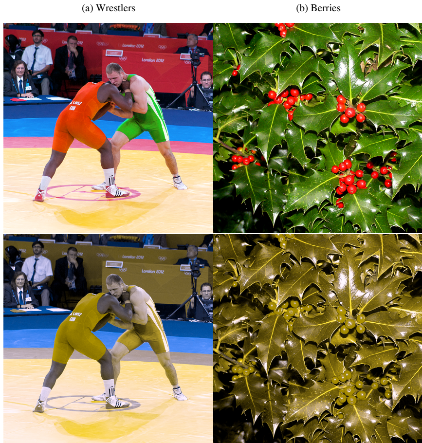
Figure 1: The first row shows the original images, while the second row shows the deutan simulations. The images have been simulated using the Brettel simulation [1].
