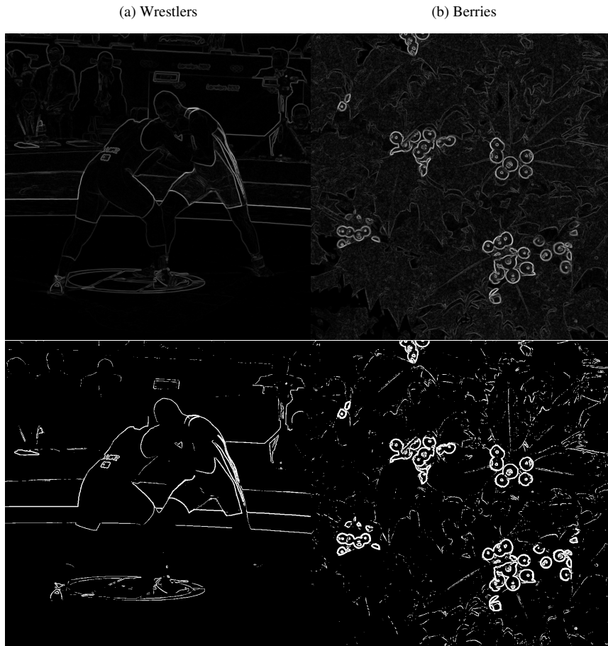
Figure 2: The first row shows the magnitude of the gradient, M . The second row shows the edge map, \mathfrak{M} , with \varepsilon = 0.15 and one round of dilation.
