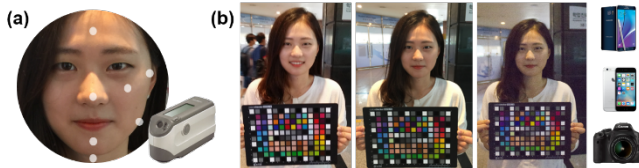
Figure 2. Structure and examples of collected dataset: (a) The L^*a^*b^* measured spots (forehead, nose-tip, chin, neck, cheek, cheekbone, jaw), (b) Images taken with three devices (Samsung Galaxy S4, Apple iPhone6, Canon 550D)
