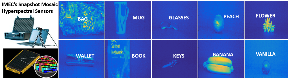
Figure 2: Proposed Hyperspectral Dataset: 10-Category Hyperspectral Image dataset, acquired by IMEC's Snapshot Mosaic Sensors.
