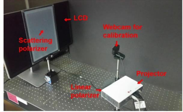
Figure 4. The experimental setup of proposed system. The scattering polarizer combines rays from the LC panel and the projector.
