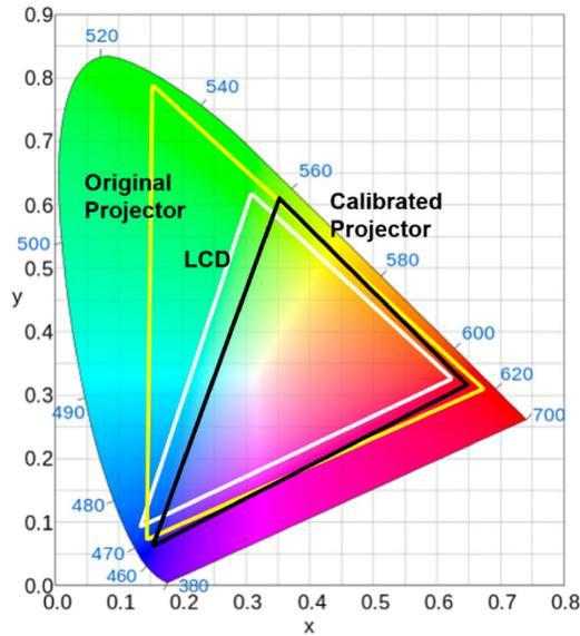
**Figure 5.** The color gamut defined by coordinates of red, green, blue in CIE  $xyY$  color space. The color gamut of the LCD is include in the color triangle of the projector. The color gamut of the calibrated projector image is more similar to that of the LCD.
