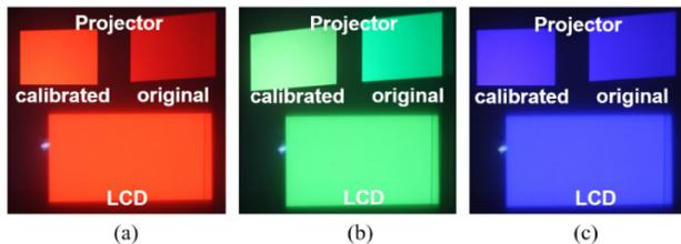
**Figure 6.** Calibrated images from the projector are compared to original projector image and LC panel image. For each picture, the images on the upper left, the upper right, and the bottom are the calibrated image from the projector, original image from the projector, and the LC panel image, respectively. Each picture represents (a) red (b) green (c) blue images.
