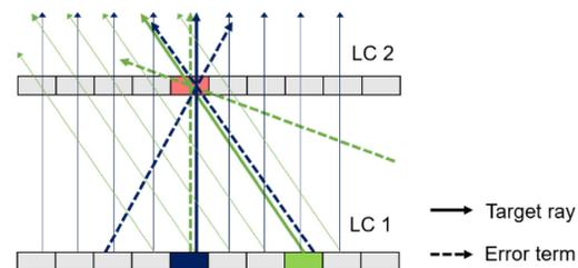
Figure 1. The principle of generating error terms caused by diffraction. The target rays are represented by solid line, and the error term is represented by dotted line.
