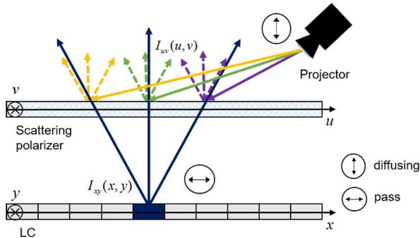
**Figure 3.** The system scheme of compressive light field display using scattering polarizer. The scattering polarizer combines rays from the LC panel and the projector.
