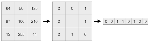
Figure 4: Left: Example 3x3 pixel neighborhood, Center: Comparison of neighbors to center pixel, Right: Local binary pattern codeword
