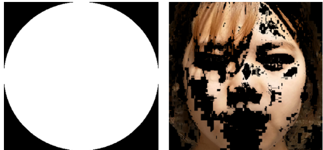
Figure 1. The pixel-based skin detection often fails because it does not discriminate nonskin regions as far as hues belonging to the predefined detection boundary. In this case, the brown hairs were detected as skin.
