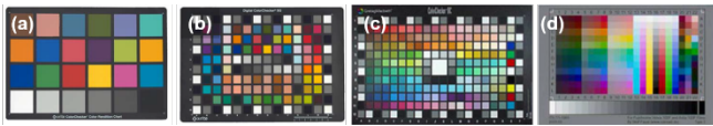
Figure 1. Examples of standard calibration targets: (a) X-Rite ColorChecker Classic; (b) X-Rite Digital ColorChecker SG; (c) Macbeth ColorChecker DC and (d) Agfa IT8.
