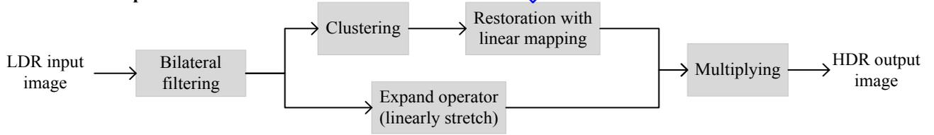
Fig. 1. Overview of the proposed iTM algorithm.
