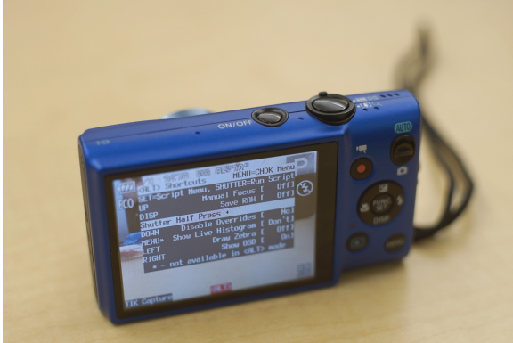
Figure 3. CHDK display with Lua script for TIK Capture loaded
