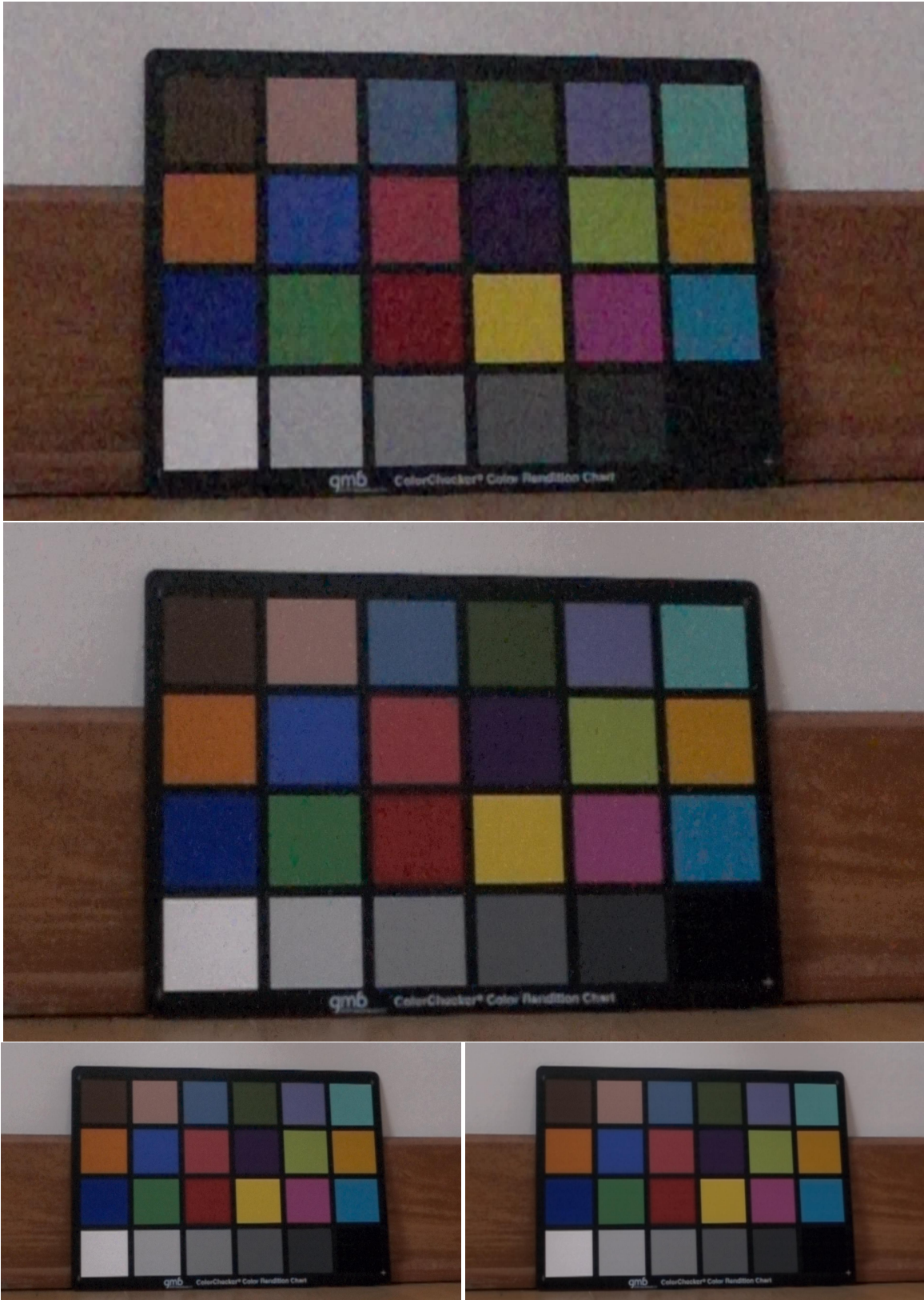
Figure 1. 960FPS frame grab from Sony RX100 IV video and TDCI virtual exposures with shutter 1/960s, 1/24s, and 1s
