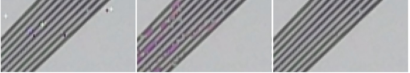
Figure 3. The result of different defect correction mechanisms for an image with simulated defects at (M_1, M_2) = (0.4, 10.0) Left: No correction, middle: median-based correction, right: proposed correction ( M_3 = 0.4 )
