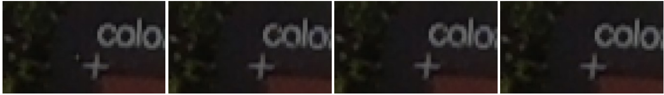
Figure 6. The result of different defect correction mechanisms for an image with real defects at (M_1, M_2) = (0.4, 10.0) Left to right: No correction, averaging-based correction, median-based correction and proposed correction ( M_3 = 0.4 )
