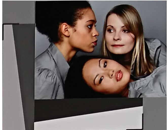
Figure 9: The bright and dark stripes along the edge and the artifacts around the girl's hair are caused by strong sharpening.
