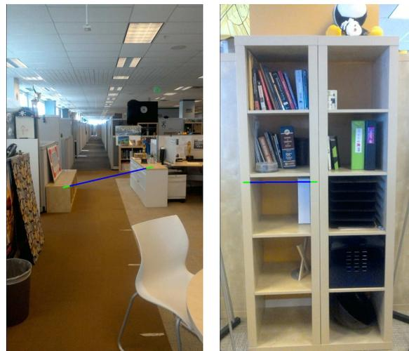
**Figure 4.** Blue line shows the line joining two points indicated by user for measurement. Green line segments show the two extensions analyzed to detect gaps.
