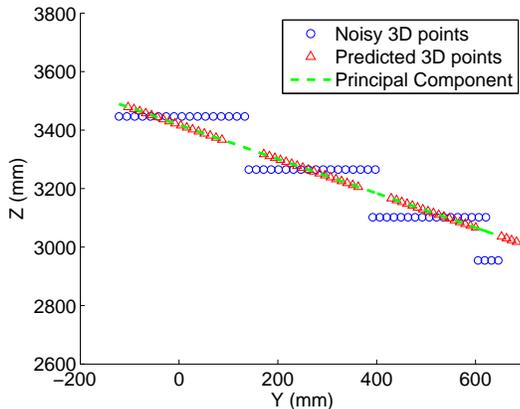
**Figure 3.** Plot showing a Y-Z slice of the 3D points resulting from the measurement in Figure 2. Blue circles show the noisy 3D points, green line shows the principal component estimated by our algorithm and the red points show the noisy points projected onto the principal component.
