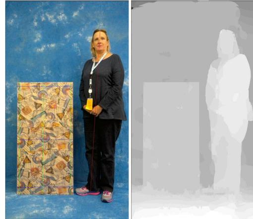
**Figure 1.** Image and co-registered disparity map from a Dell Venue 8 tablet. Disparity inaccuracies are visible along the edges of the target board, especially along the bottom edge. These will result in measurement inaccuracies when the user selects points in these areas to measure the dimensions of the target board.
