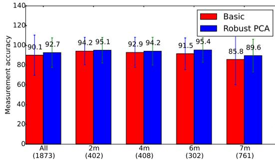
**Figure 5.** Measurement accuracy using our method. The “Basic” algorithm uses the median disparity in a window centered around each point for triangulation. The numbers in parentheses under each bar represent the number of data points in each category.
