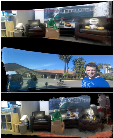
Figure 3. Examples showing failure cases of traditional methods. From top to bottom: perspective distortion in the sofa on the right side (2D stitching), ghosting artifact due to a moving person on the left side (2D stitching) and low RGB fidelity on the right side (3D stitching).
