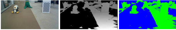
Figure 5. Hybrid 2D/3D approach (left to right): a frame from the ‘Penguin1’ sequence, disparity map, map indicating 2D and 3D parts in the hybrid scheme. Far objects and near objects with unreliable depth estimates (blue regions) are being fed to the 2D pipeline.
