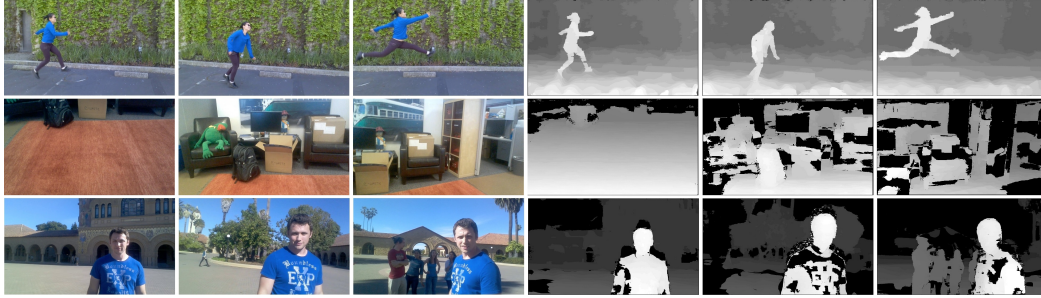
Figure 4. Some frames and disparity maps from our typical input sequences. Top row: ‘Jump’ sequence (handheld panning camera following a fast moving object), Middle row: ‘Penguin2’ sequence (static scene with challenging surfaces for depth, rotating camera), Last row: ‘Stanford selfie’ sequence (scene with moving objects within and outside camera depth range, handheld camera rotating nearly 360 degrees).
