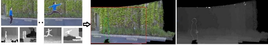
Figure 1. Overview of the proposed method which uses RGB-D and object segmentations to output a clean RGB-D panoramic scene. The red box denotes the first frame and the green outline shows the moving object in the reference frame.
