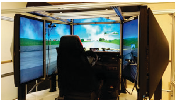
Figure 1. A wide field VR environment driving simulator (FAAC Inc. Ann Arbor, MI) used to induce motion sickness.
