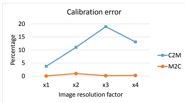
Figure 11: Percentage of the average error for applying camera calibration algorithms to the images extracted by the C2M and M2C methods for various resolutions.
