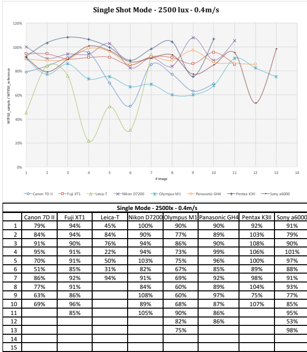
Figure 12. AF Tracking Single Shot Mode - The camera captures images in single shot mode while the object is moving with 0.4m/s from far position (5m) to near position (2m). Graphical and numerical results for 2500lux illumination.
