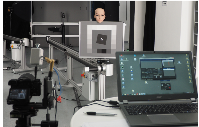
Figure 9. AF Tracking measurement setup. The DUT on the left, pointing at the test target mounted on a moving stage. The track length of the stage is 3m, resulting in a maximum distance of 5m and a minimum distance of 2m. The chart moves diagonal to the optical axes. An artificial face is mounted on top of the chart, the measurement is performed on the slanted edges of the test chart. A mechanical finger released the camera, synchronized with the moving stage.
