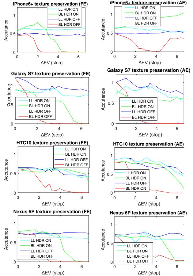
**Figure 9.** Texture preservation measurement results for 4 devices (from top to bottom: iPhone 6+, Galaxy S7, HTC 10, Nexus 6P). The first column shows the result with exposure forced on the left DMX texture. The second column is the result with auto exposure. The abscissa is the difference of luminance between the two DMX in photographic stops.
