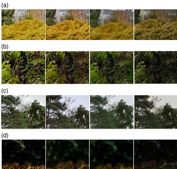
**Figure 17.** Natural HDR scene. (a) HDR scene shot with the Galaxy S7. (b), (c), (d) and (e), from left to right: Galaxy S7, Nexus 6P, HTC 10 and iPhone 6+. Compared to the sky, (b) has 2 stops of luminance difference, (c) and (d) have 4 to 5 stops of luminance difference, (e) has 7 stop of luminance difference.
