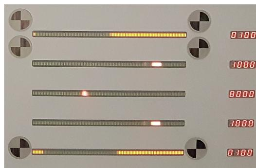
**Figure 13.** Ghost observed during classic timing measurement. Exposure time is computed by counting the number of lit LEDs. As the LEDs are lighted on and off at a known speed, we can deduce the resulting exposure time. Thus Ghosting can result in a wrong exposure time.
