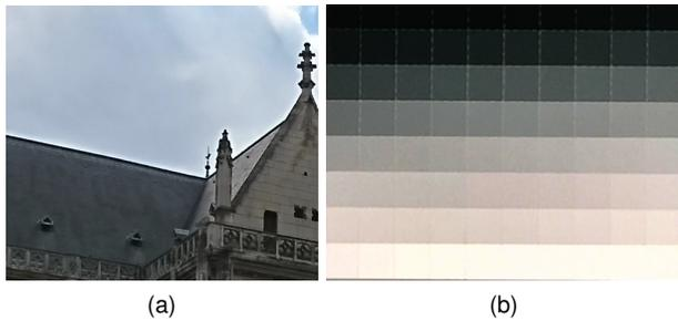
**Figure 5.** (a) is an example of halo artifacts between the roof and the sky, which can be reproduced by our setup (b). The homogeneous patches are brighter on their upper edge than on their lower edge.
