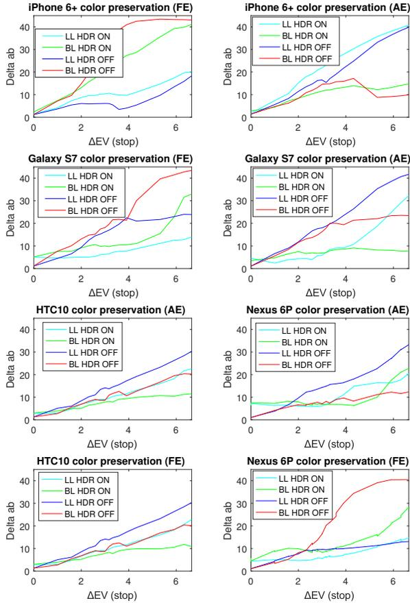
**Figure 10.** Color preservation measurement results for 4 devices (from top to bottom: iPhone 6+, Galaxy S7, HTC 10, Nexus 6P). The first column shows the result with exposure forced on the left DMX texture. The second column is the result with auto exposure. The abscissa is the difference of luminance between the two DMX in photographic stops.
