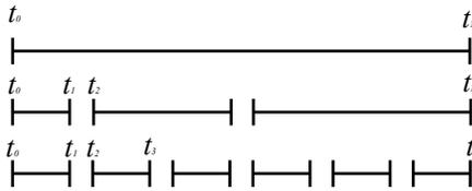
**Figure 15.** The exposure time of a traditional single-image device (represented as a line in the first row) can be used by a multi-image device to allocate multiple exposures in different ways (second and third rows).
