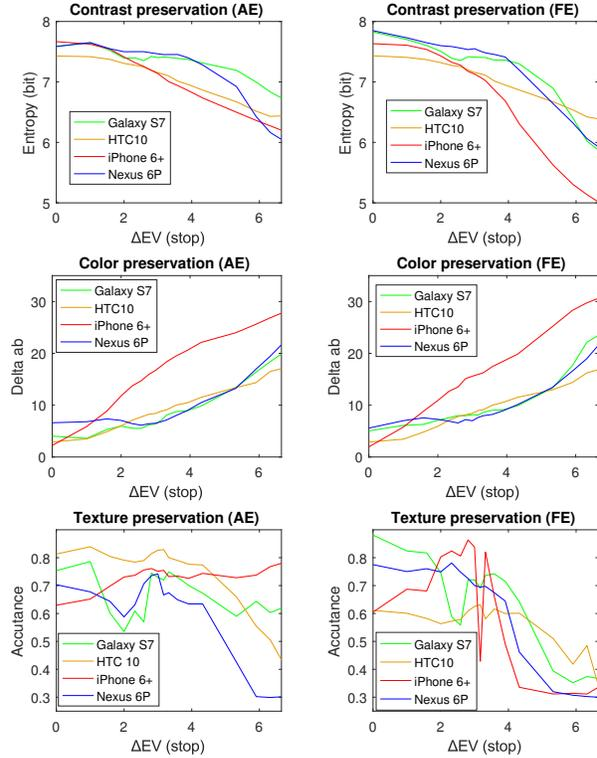
**Figure 16.** Results of the HDR setup for the Galaxy S7 (green), HTC 10 (orange), iPhone 6+ (red) and Nexus 6P (blue). Each measurement is computed as the mean of the measurement of the bright light DMX and the low light DMX on HDR ON picture. The abscissa is the difference of luminance between the two DMX in photographic stops.
