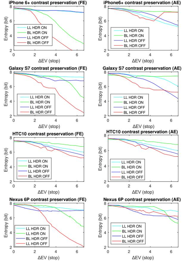
**Figure 7.** Local contrast preservation measurement results for 4 devices (from top to bottom: iPhone 6+, Galaxy S7, HTC 10, Nexus 6P). The first column shows the result with exposure forced on the left DMX texture. The second column is the result with auto exposure. The abscissa is the difference of luminance between the two DMX in photographic stops.
