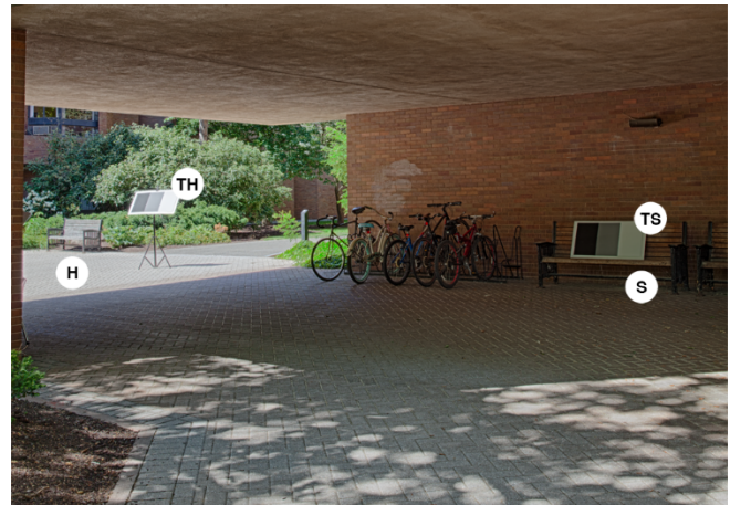
Figure 3. Measurement Map TH = Target in Highlights TS = Target in Shadows H = Adopted Highlights S = Adopted Shadows
