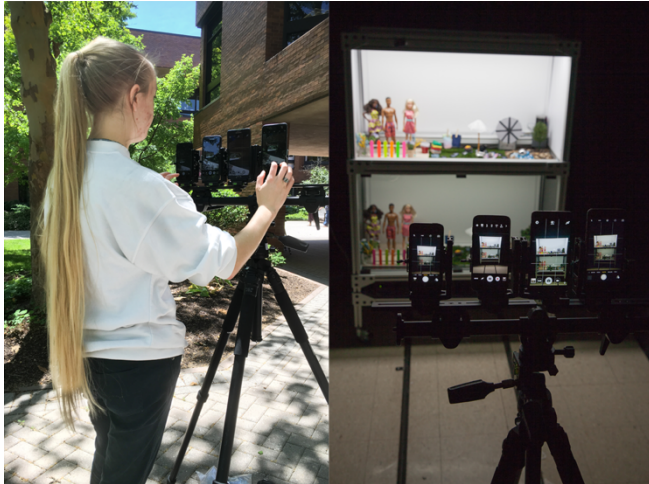
Figure 4. Capturing Scenes Image A – Capturing natural exterior scene using four different mobile phones Image B – Capturing laboratory scene using four different mobile phones
