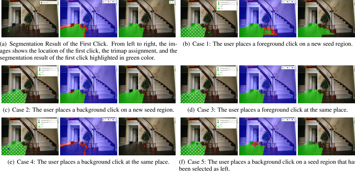
Figure 6. An Example of Trimap Assignment for the Second Click. The example shows the second click followed by the first click showed at (a). Each case from the left to right shows the new seed region, the Trimap assignment, and the segmentation result. (a) The first left click selects the tiled floor. (b) A foreground click is placed at a region that doesn't belong to previous seed region highlighted in dot pattern. (c) A background click is placed at a region that doesn't belong to previous seed region highlighted in dot pattern. (d) A foreground click is placed at the same location as a previous background click. (e) A background key is placed at the same location as a previous left click. (f) A background key is placed at a selected seed region which was selected by a left click before.
