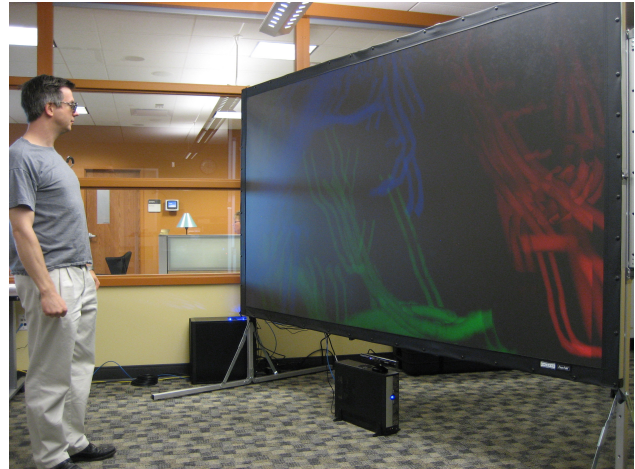
Figure 5. Tracked user in front of the passive projection screen with the tracking computer and the Kinect sensor on top underneath the screen.
