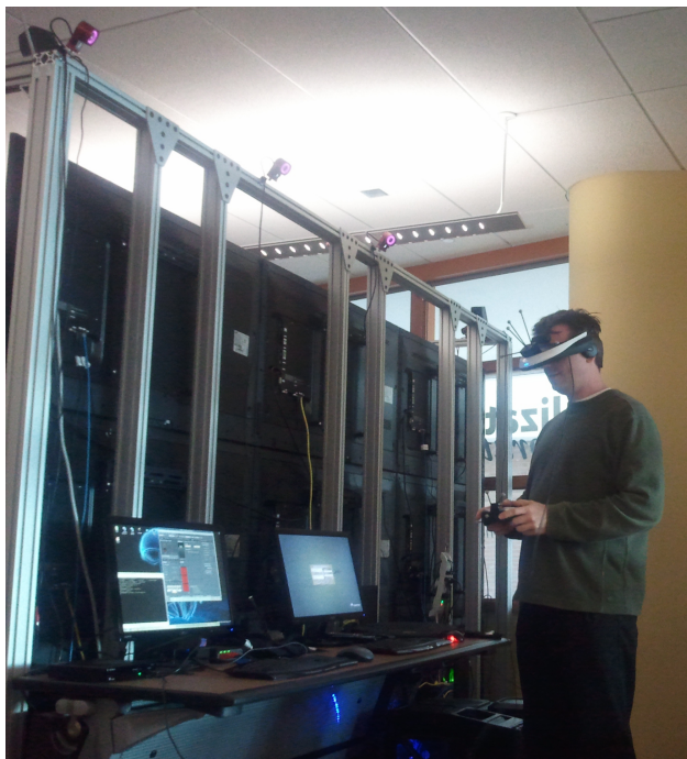
Figure 8. User wearing a head-mounted display. Head position and input device are tracked via the optical tracking system mounted on the aluminum framing (top left).
