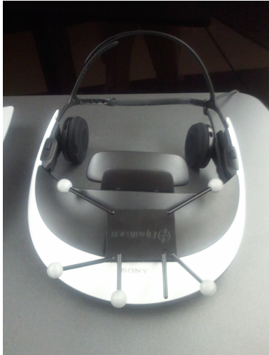
Figure 7. The Sony HMZ-T1 head-mounted display with reflective markers attached for tracking.
