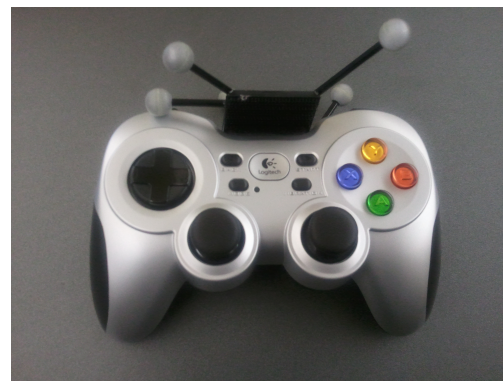
Figure 9. Logitech gamepad with reflective markers attached for tracking.
