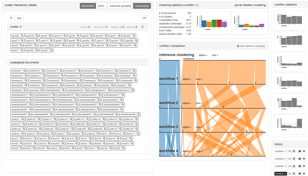
Figure 4. Clustering Comparison View: Workflow statistics panel (right): F -measure (if reference clustering is available), computation time, average separation, average compactness, Dunn and Davies-Bouldin indexes of different clusterings can be compared. Cluster statistics panel (top): clustering statistics of workflow on top of cluster comparison panel are shown. Workflow comparison panel (middle): clustering results (rows) are separated into clusters according to underlying document counts; order of clusterings can be adapted via drag-and-drop; color of bands represent clusters of clustering on top; band width represents number of documents in band. Cluster intersection panel (left): shows documents within a band selected in the cluster comparison panel; alternatively, most frequent or correlated terms can be shown. History panel (bottom right): created workflows are represented by ID, latest workflow step, copy and delete buttons; current workflow is highlighted, via the check boxes users can select workflows to be compared.
