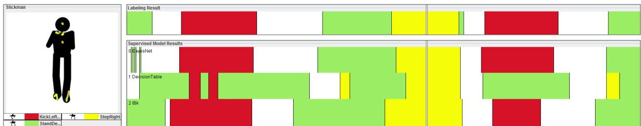
Figure 6. Labeling support by supervised algorithmic models. An interface allows adding classifiers learning the use-based labels. The results of the classifiers can be visually compared. In the example a boxing pose is shown, the yellow label represents an upright stand. Three classifiers are tested with the current MoCap sequence. It can be seen that BayesNet and IBk fairly match the labeling, while the DecisionTable produces a bad classification result.
